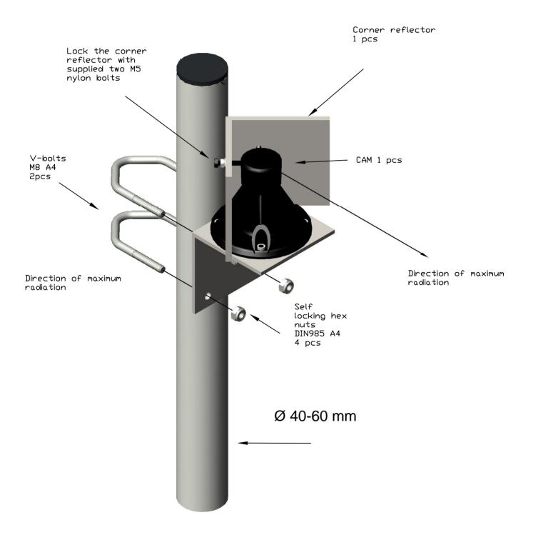
For proper weather protection all connectors and cable junctions should be covered by self-amalgamating tape or equivalent
